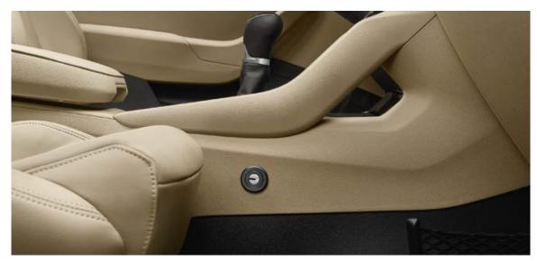
Mechanical transmission locking system for LHD
